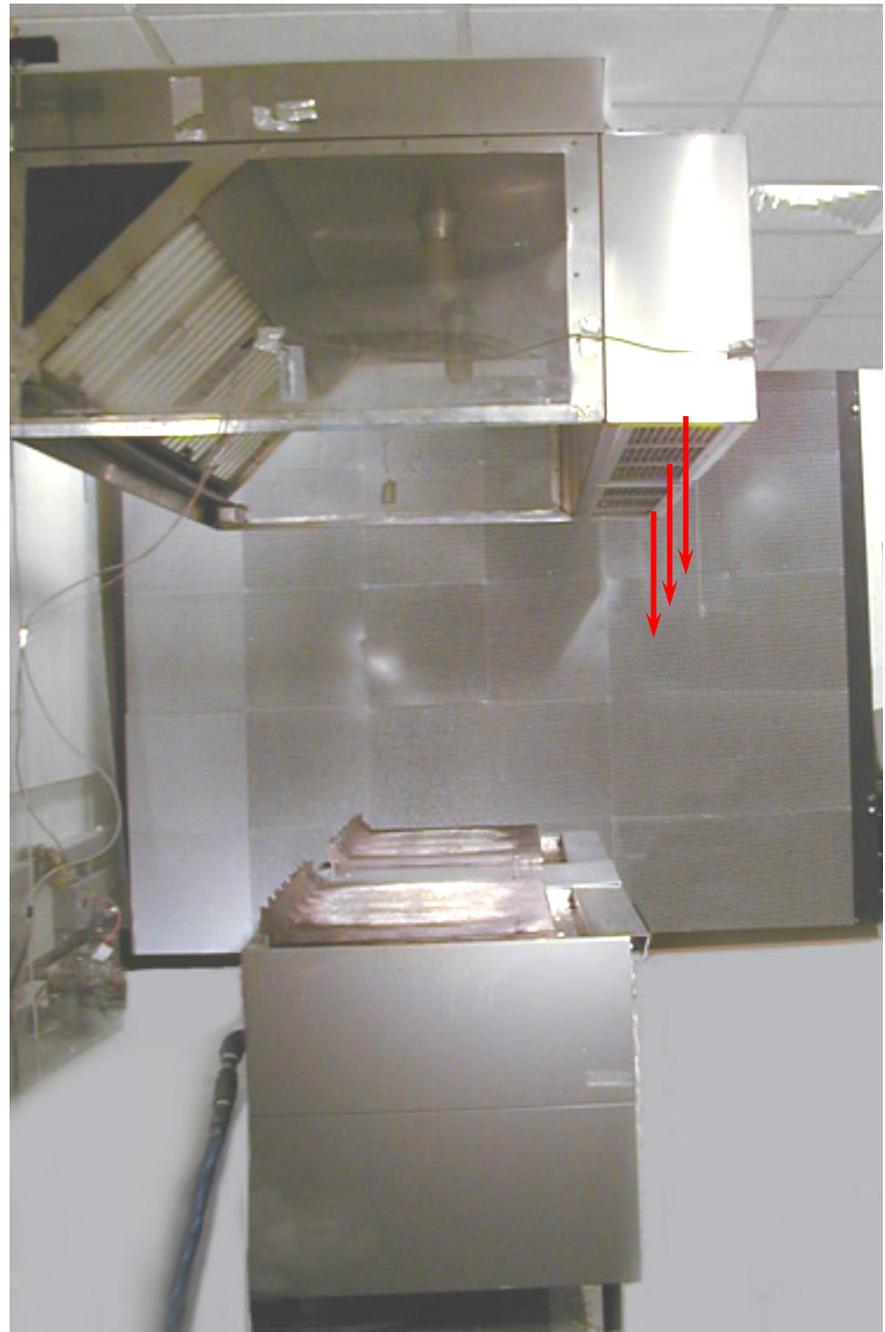
Two Broilers Simulated Cooking -- Spillage at 4100 cfm
